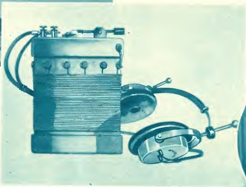
Paper clips, an old cheese box, wire, a crystal and ear-phones: That's all you needed to build a radio receiving set in 1920
